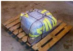
*Yes – Engine leak free, tightly shrink wrapped and well secured to pallet base*
