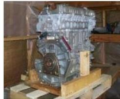
*Yes- Machine, leak free and well secured to a bespoke pallet*
