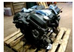
*No – heavy engine not secured efficiently to a pallet base (plastic banding is not enough)*
