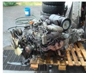
*No – awkward shape not on a bespoke pallet, not secured to pallet base*
